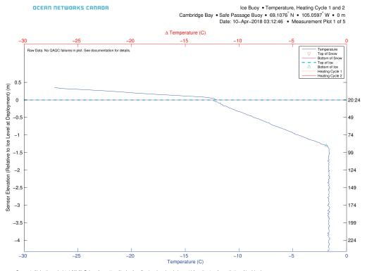
Comments: No heating cycle data (all NaN). Bottom of snow / top of ice locations (lines) are based on deployment information, top of snow / bottom of ice (triangl markers) are from the snow/ice thickness derived sensor values.
