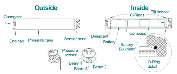
*The figure above shows a standard Aquadopp, and particular models can vary from the above. The list below describes the major system components.*
