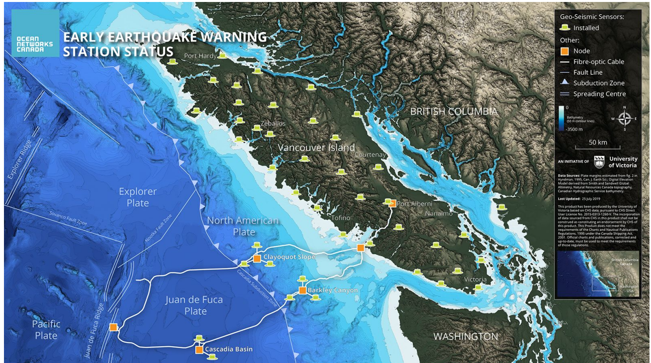
Figure 1: A high-level view of the final earthquake early warning system network, where fully installed stations are indicated by a green symbol.
