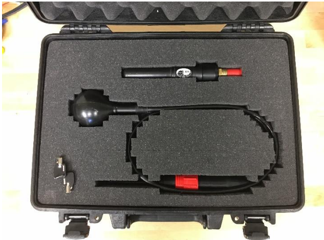
Figure 5-5 Reference hydrophone and projector
