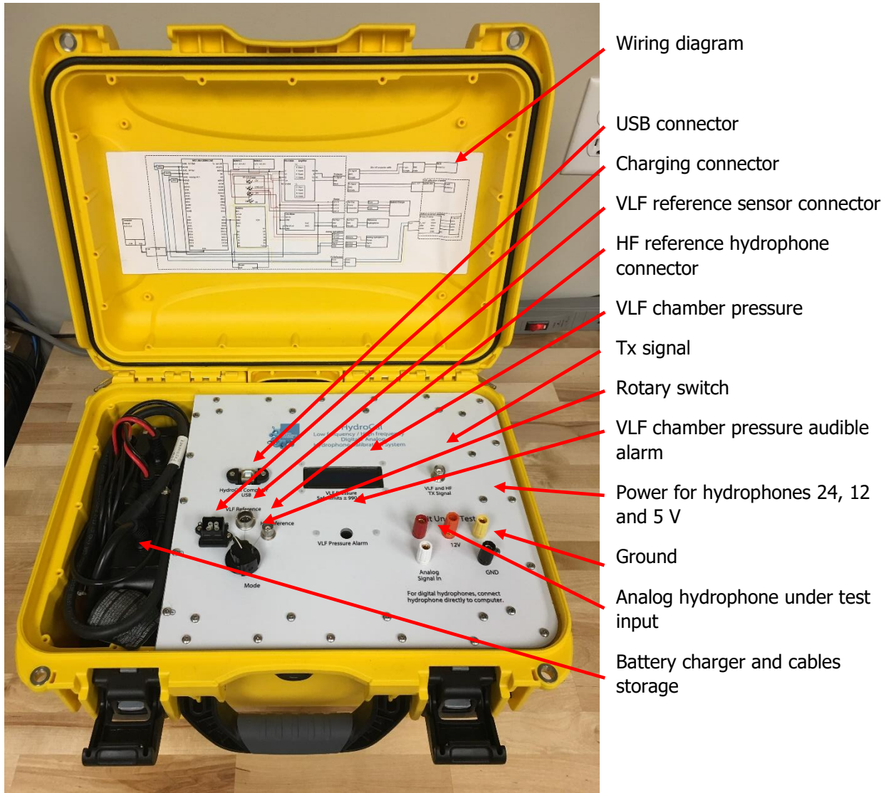
Figure 4-3 HydroCal Case Interface
