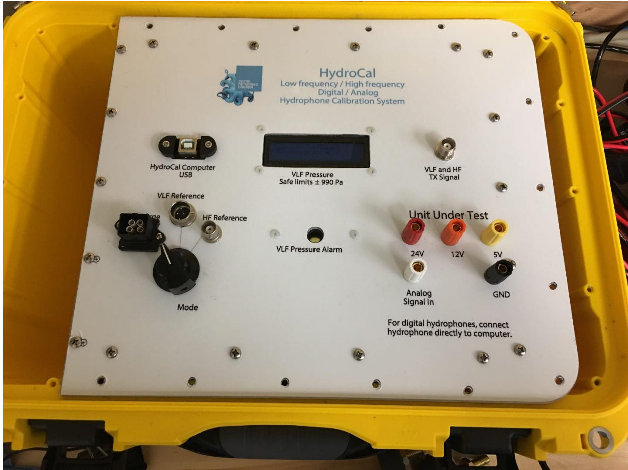
Figure 5-6 Slide the face plate to the left prior to lifting from the case.
