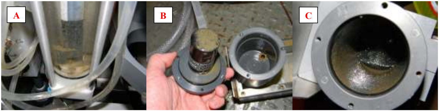
Figure 2. Pictures of each instrument: A) SBE Thermosalinograph; B) Aanderaa optode and housing; and C) view looking down the BBFL2 housing; note that the instrument measuring face is the bottom surface. These photographs were taken on the most recent maintenance trip (July 18, 2014) and clearly indicate the potential for sediment accumulation and bio-fouling taking place in just 2 weeks following the previous cleaning (July 4, 2014).
