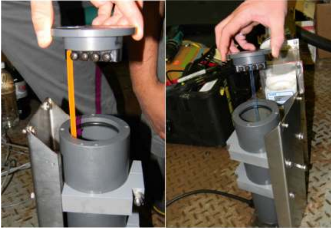
Figure 3. Photographs of pink (left; appears orange with camera flash) and blue fluorescent sticks held in place on the end-cap bracket. The relative location along the bracket and position of the end cap was kept constant and corresponds to a mid-range fluorescent reading.
