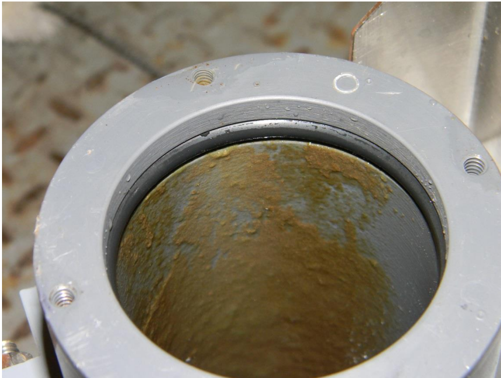
Figure 10: Biofouling within BBFL2 unit.
