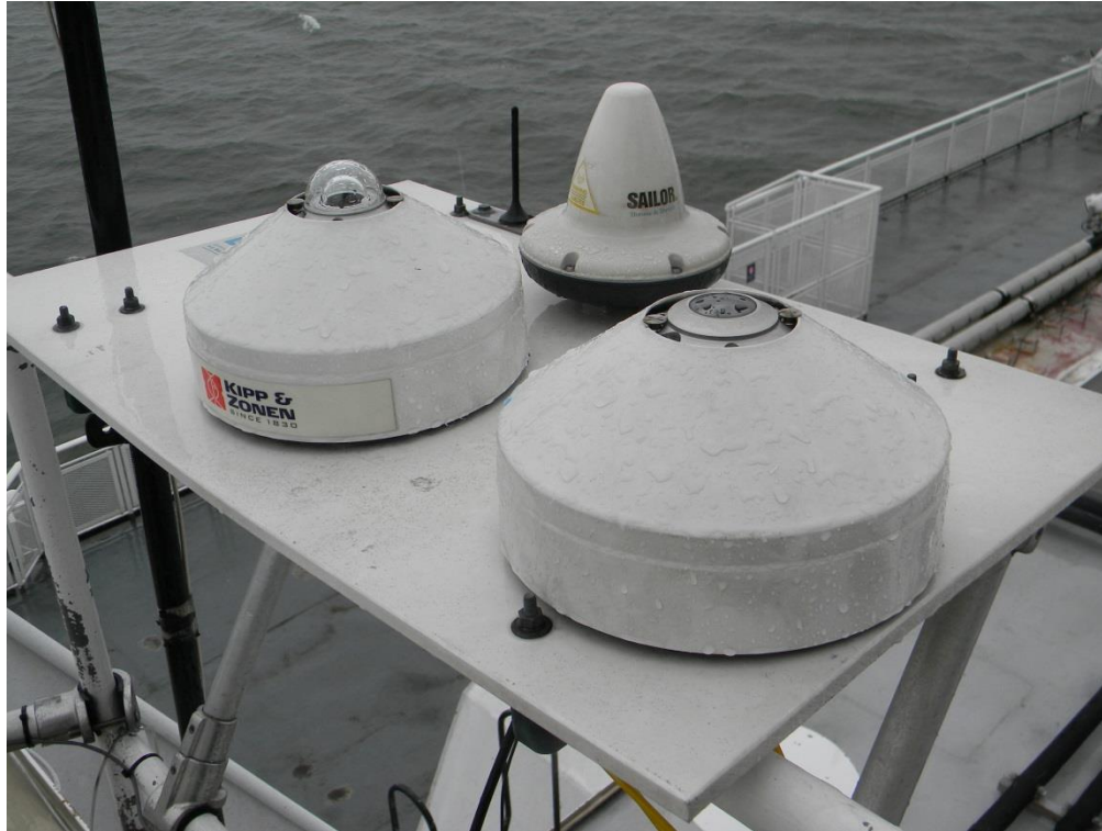
Figure 13: Radiometer and Pyranometer as remounted.
