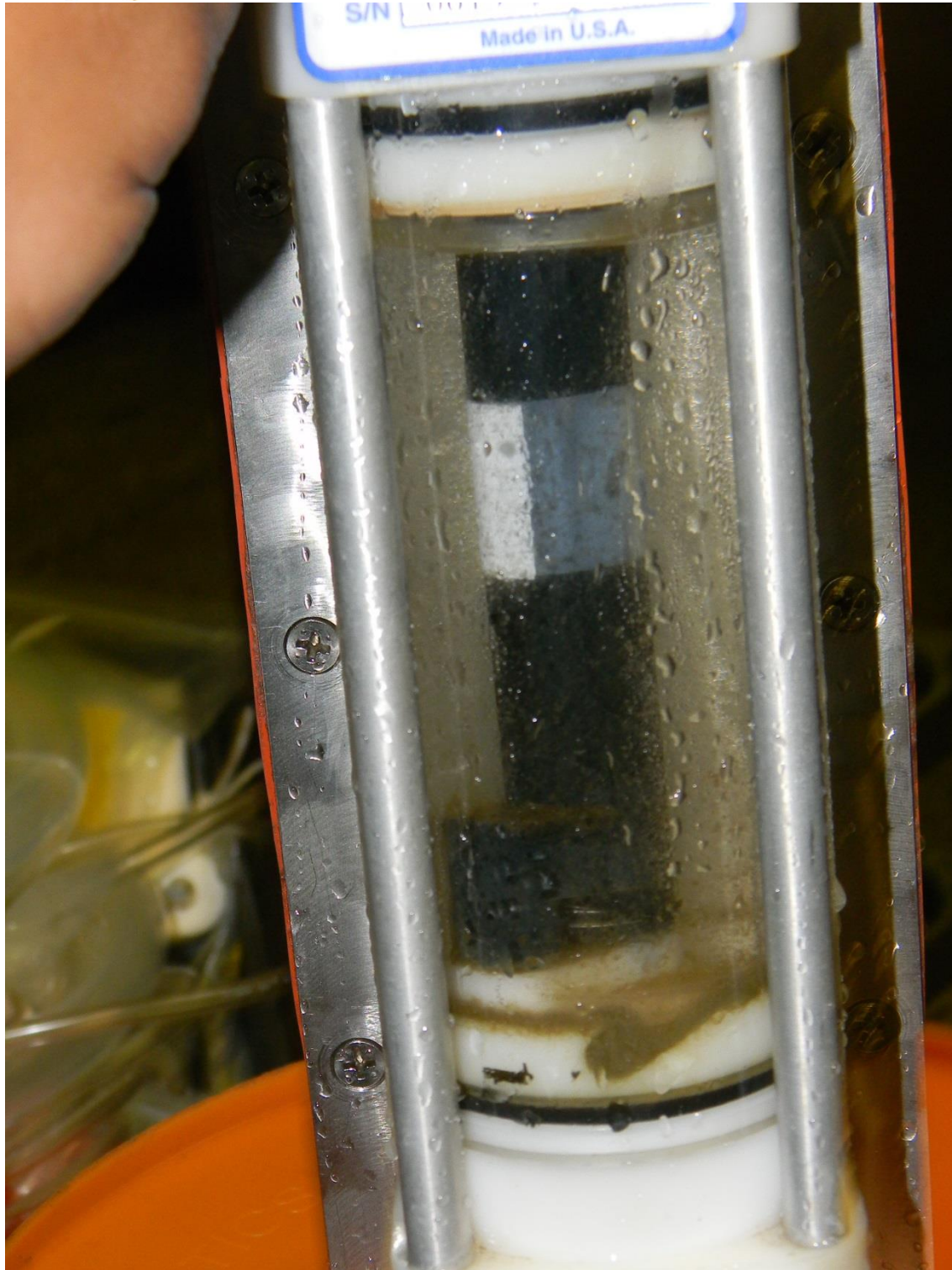
Figure 6: Sedimentation/biofouling within CT unit.
