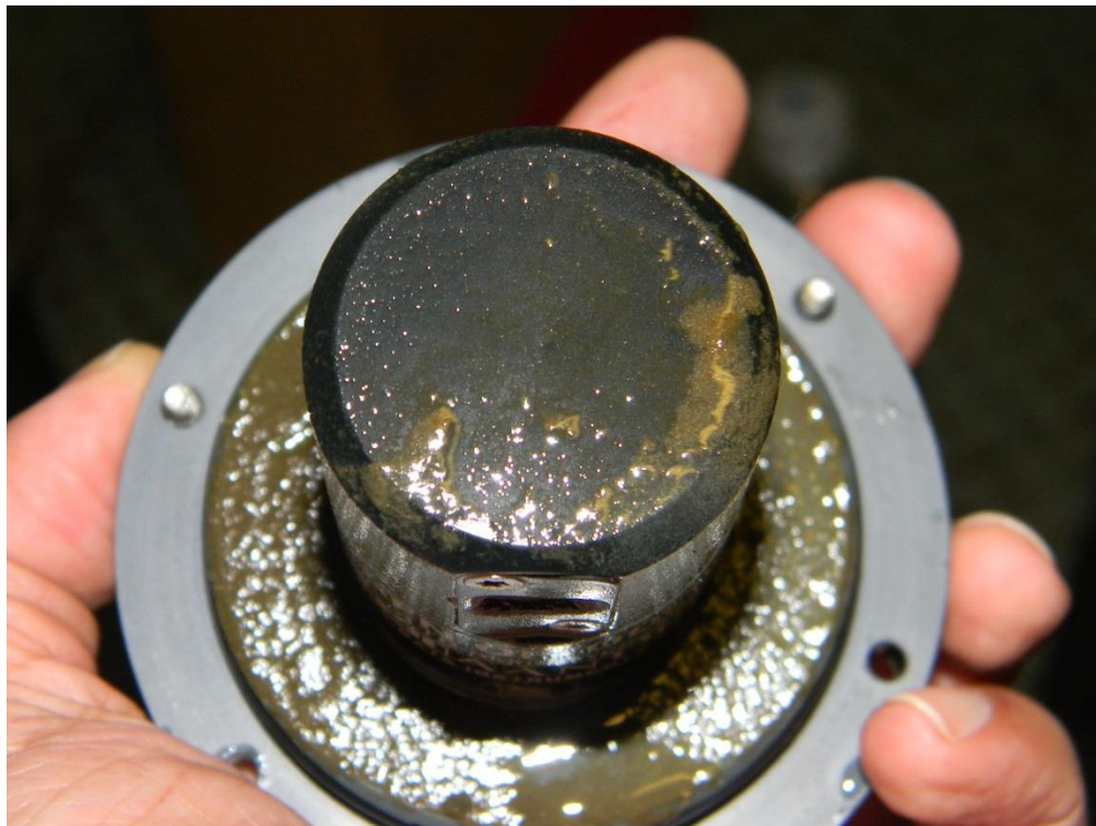
Figure 8: Biofouling on OPTODE unit.
