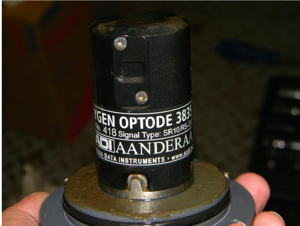
Figure 7: Biofouling on OPTODE unit.
