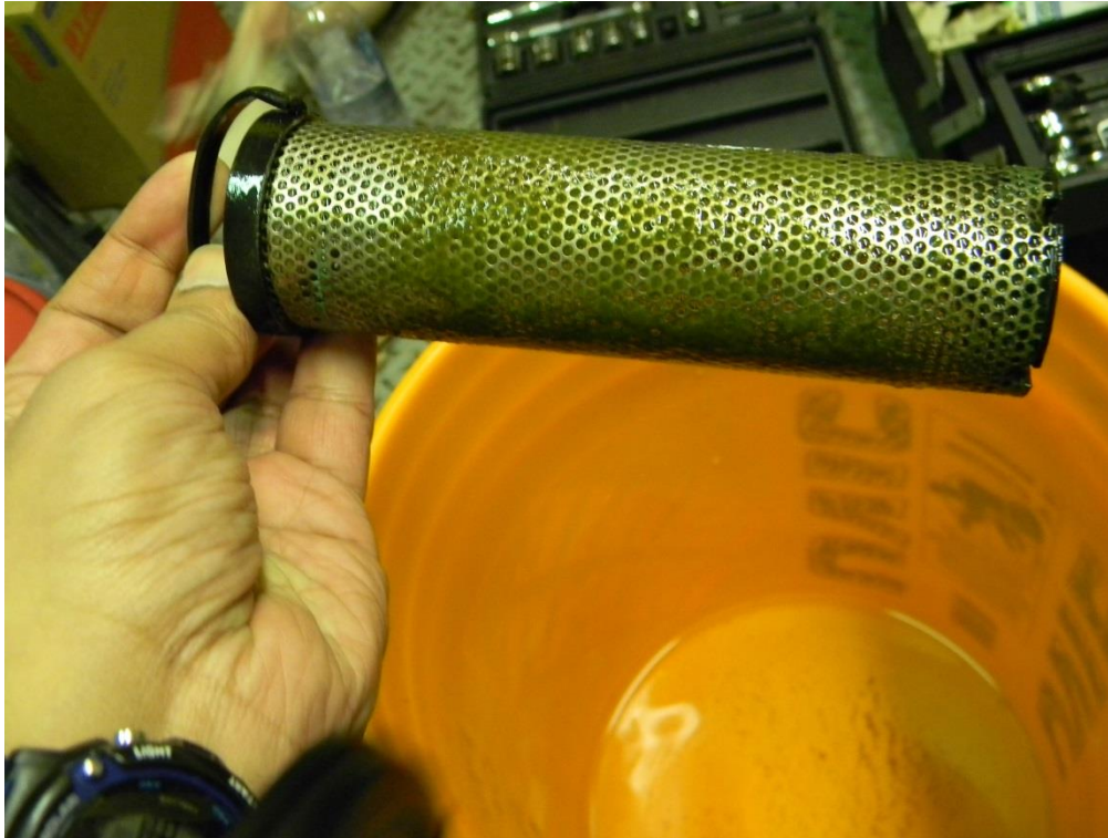
Figure 11: Biofouling of Sea Strainer.
