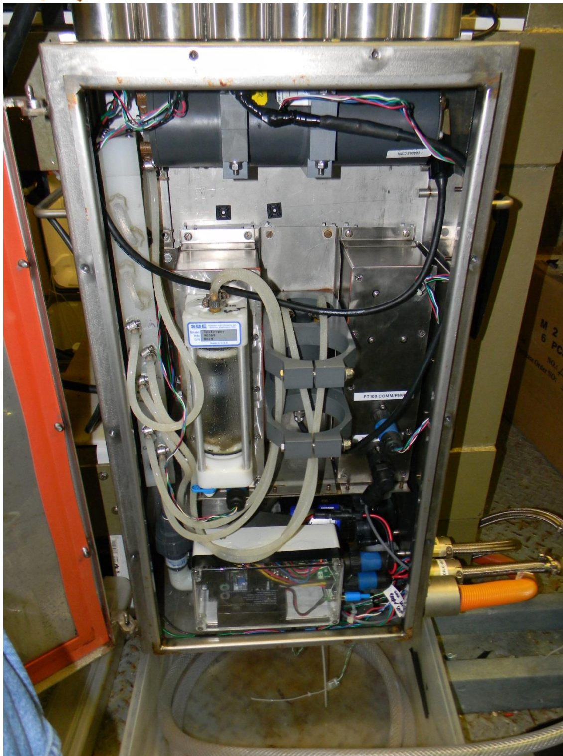
Figure 1: Instrument Box upon arrival. Note condensation throughout. Note dry catchment basin.
