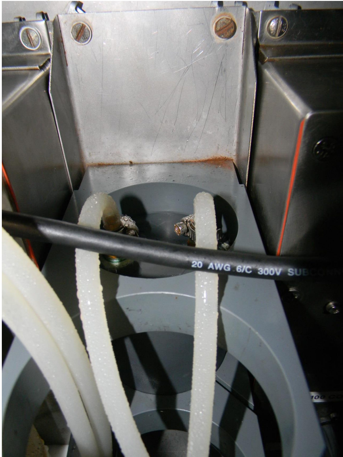
Figure 5: Condensation on OPTODE unit.
