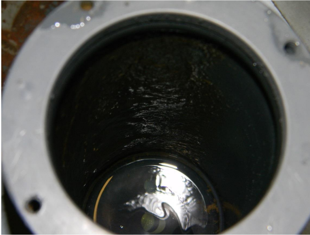
Figure 9: Biofouling within BBFL2 unit.
