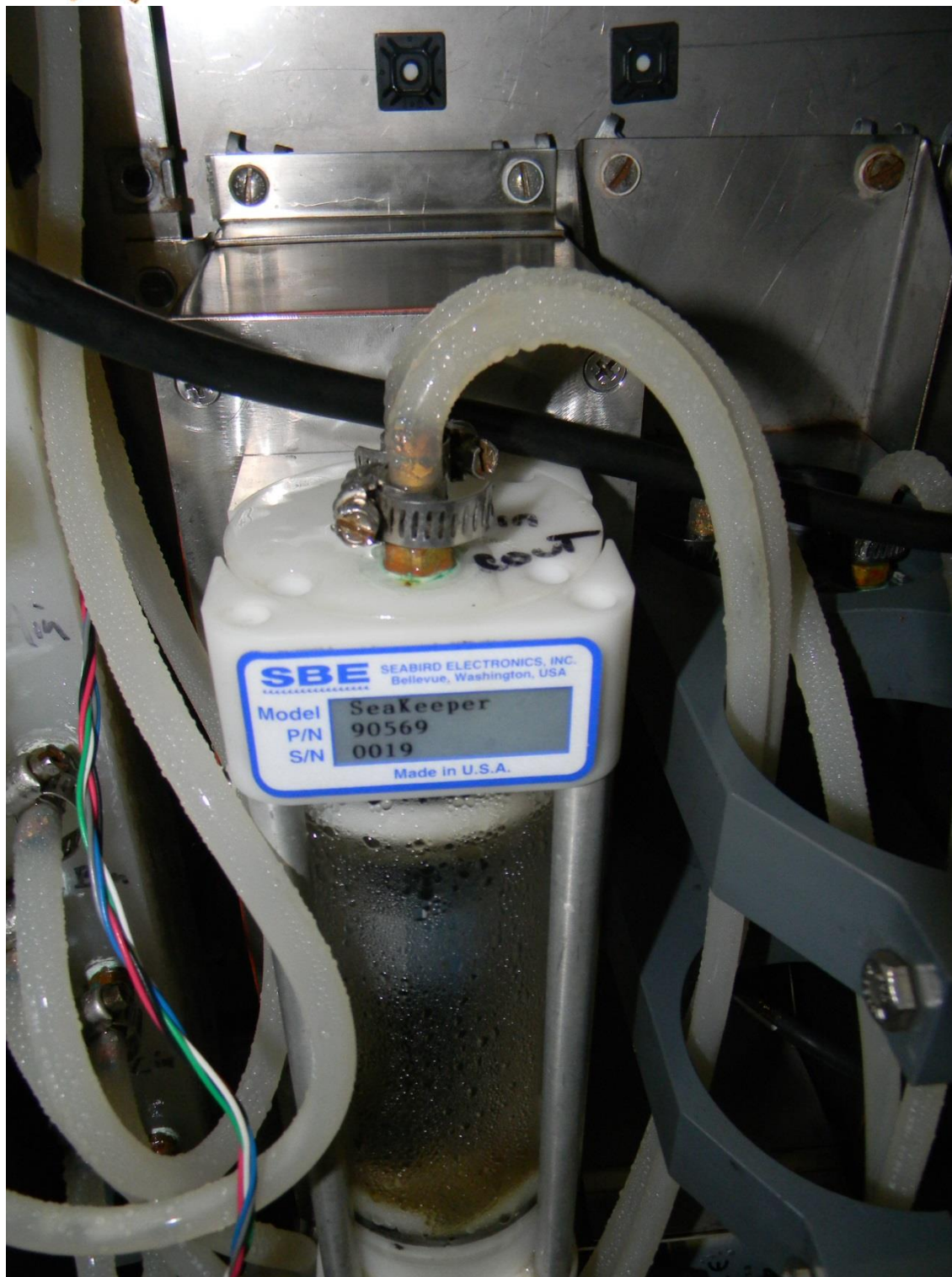
Figure 4: Condensation on CT unit.
