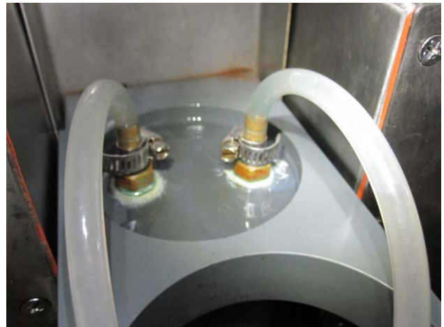
Figure 3 - water pooling on optode
