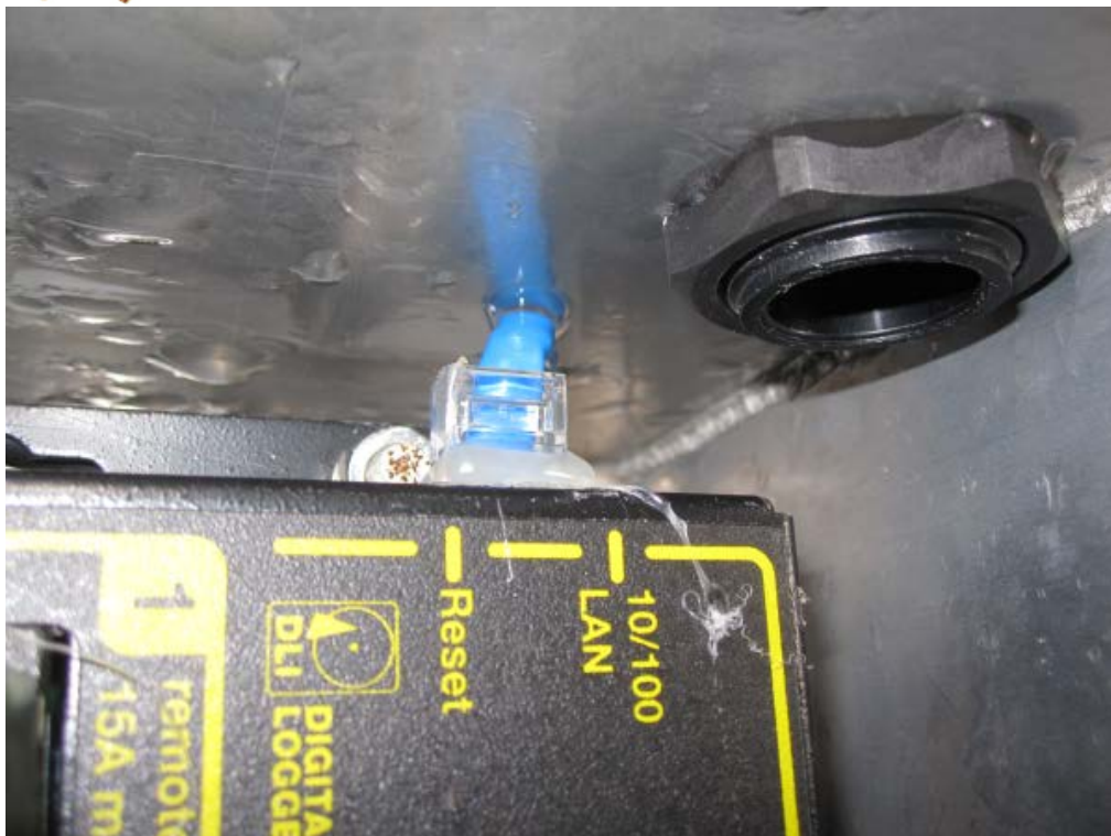
Figure 5 - topside box - right side vent and ethernet port on Web Power Bar pictured
