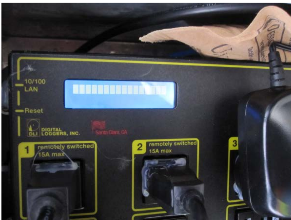
Figure 6 - Web Power Bar has entered a non-recoverable failure mode
