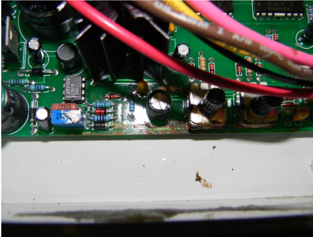
Figure 14: Pump Control board corrosion after rudimentary cleaning
