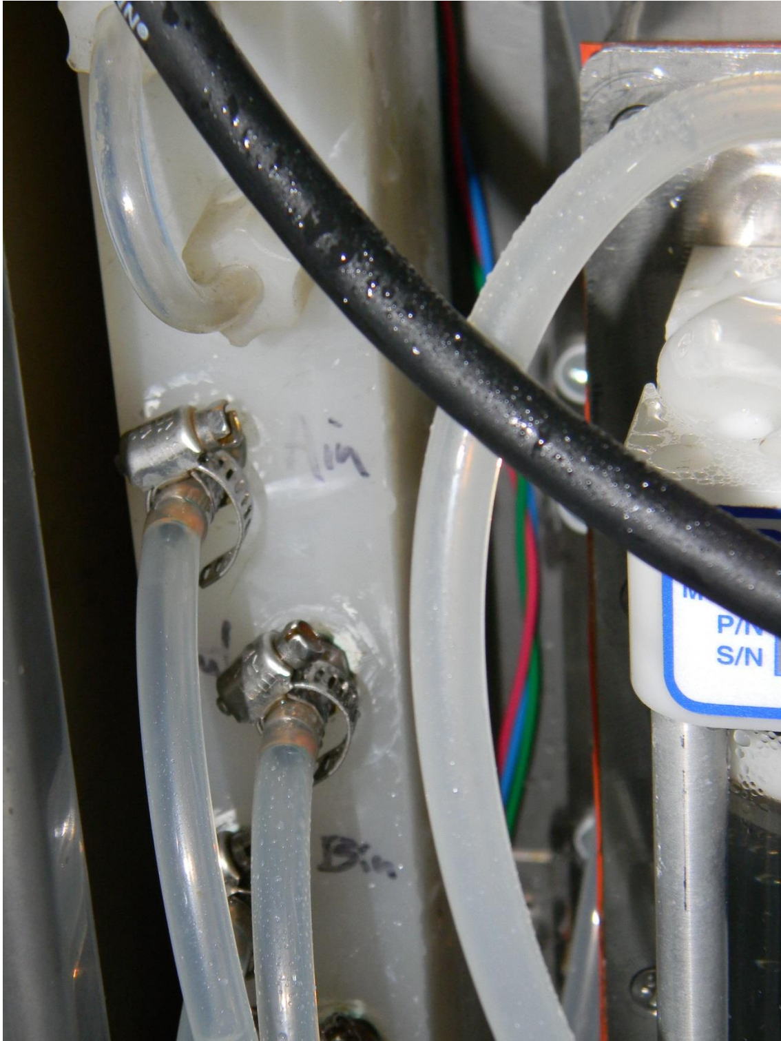
Figure 2: Water Spray on Manifold
