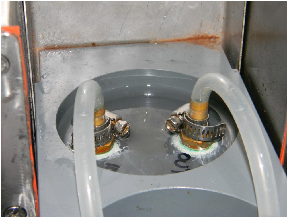
Figure 1: Water pooled in top recess of Optode
