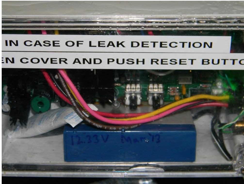
Figure 6: Pump Control Box. Note water pooled inside front edge of housing, plus visible corrosion products at junction of battery and board. Desiccant package was fully absorbed.
