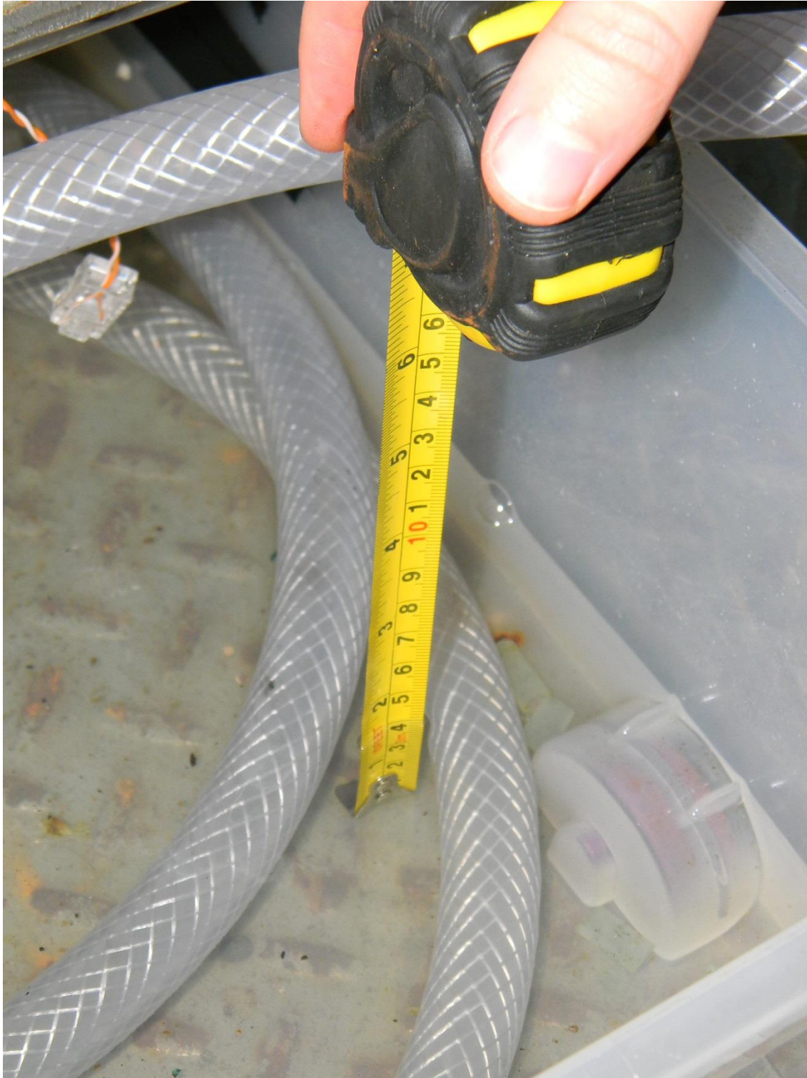
Figure 7: Depth of water within the catchment basin (approximately 4 cm)
