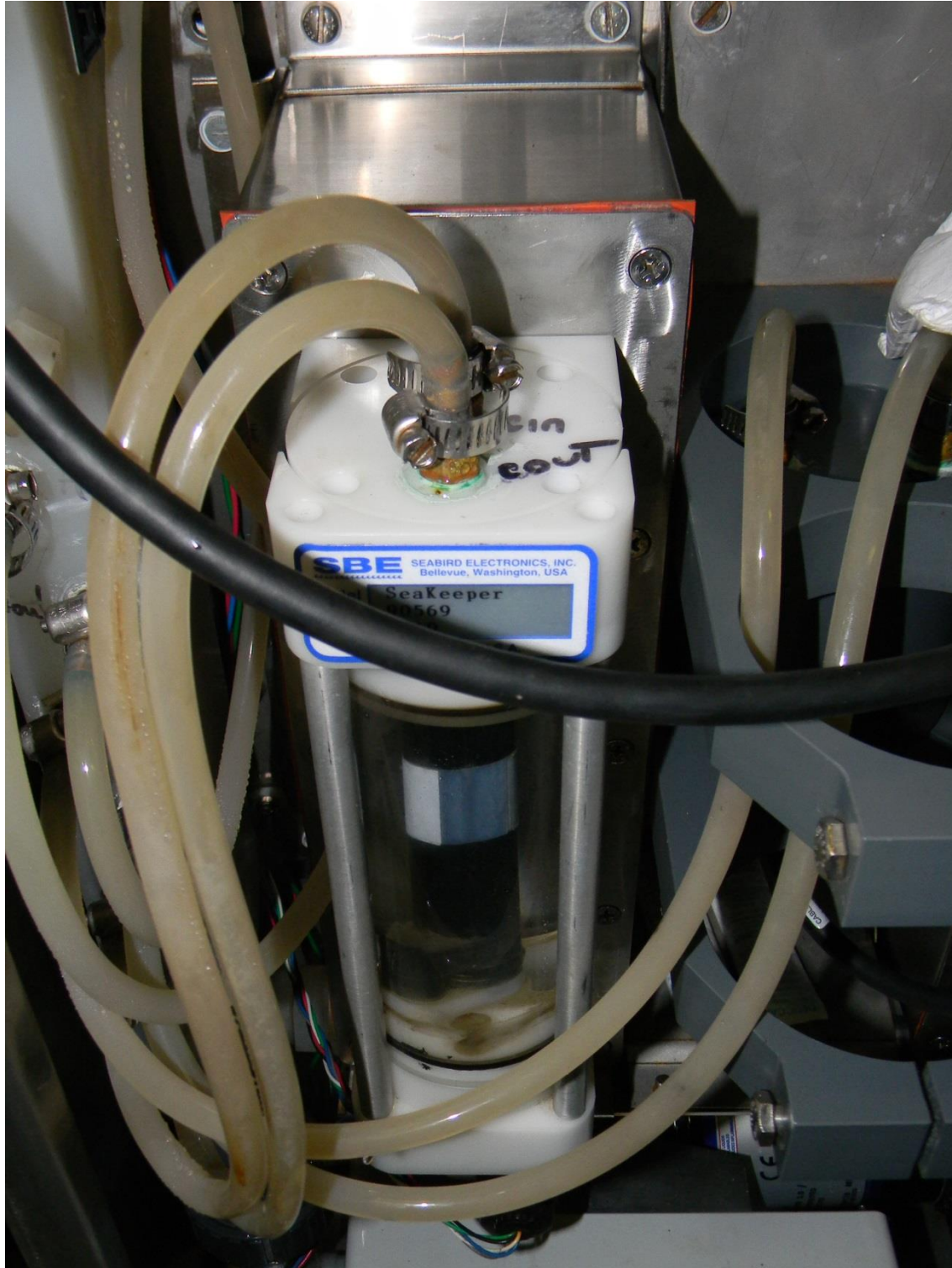
Figure 2: CT Unit. Note condensation on tubing
