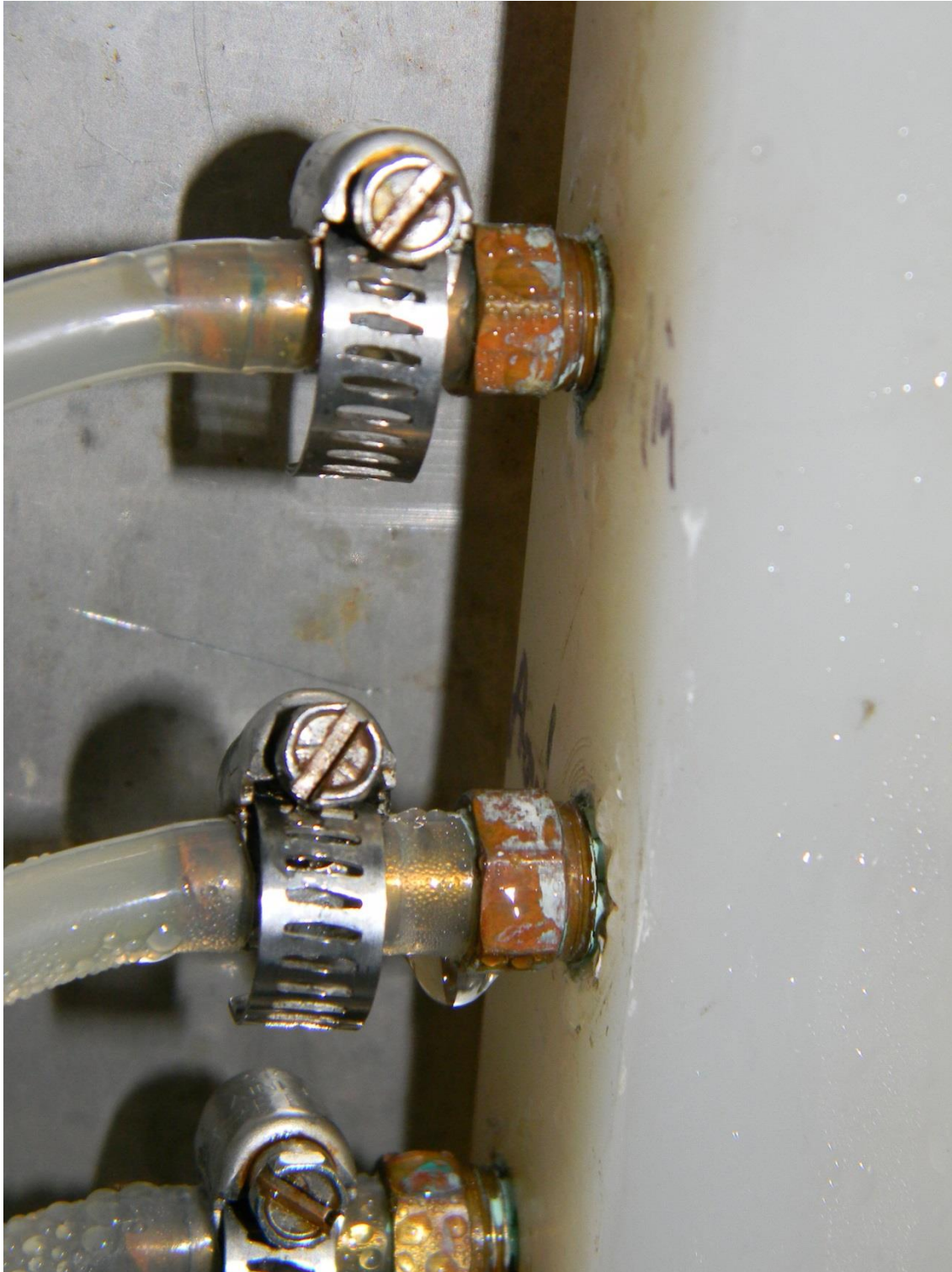
Figure 6: Correctly and incorrectly install hose clamps. The top clamp has been reinstalled correctly (set as close to the base of the barb as possible, snug without serious deformation of the rubber). The bottom clamp is set too far toward the end of the barb.
