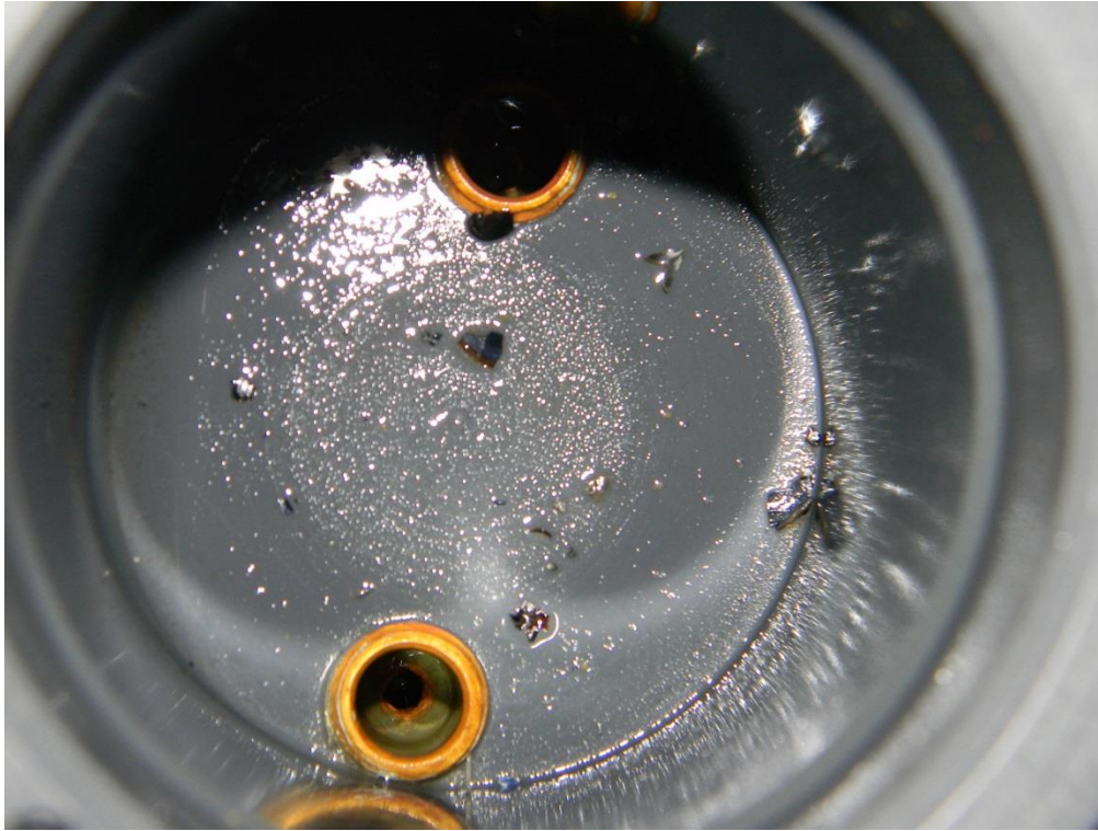
Figure 8: Sediment within the OPTODE housing.
