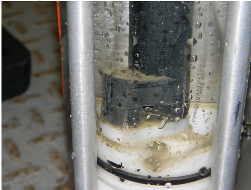
Figure 4: Fouling in the CT unit.
