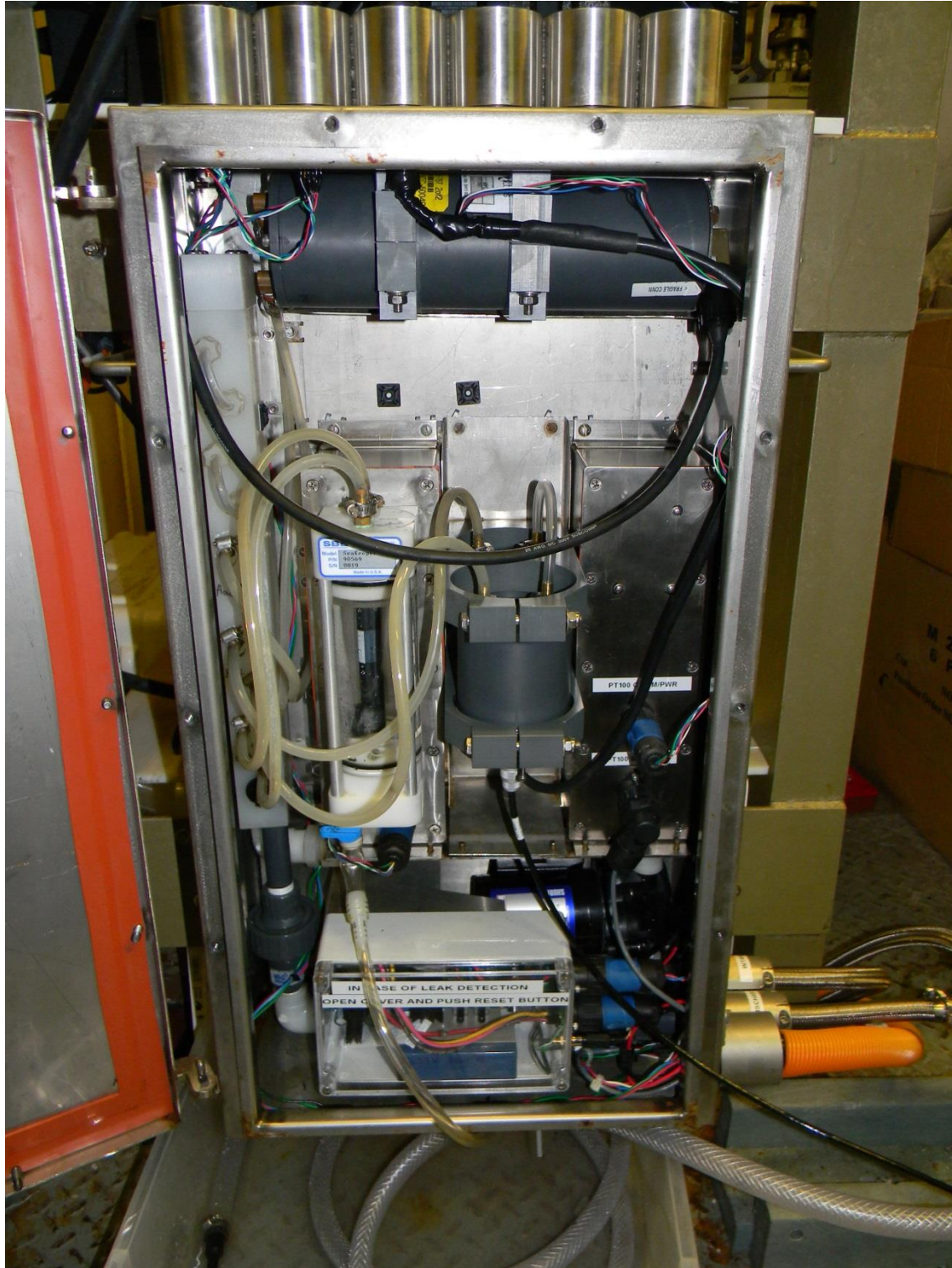
Figure 16: Temporary double-OPTODE and sample tube setup.
