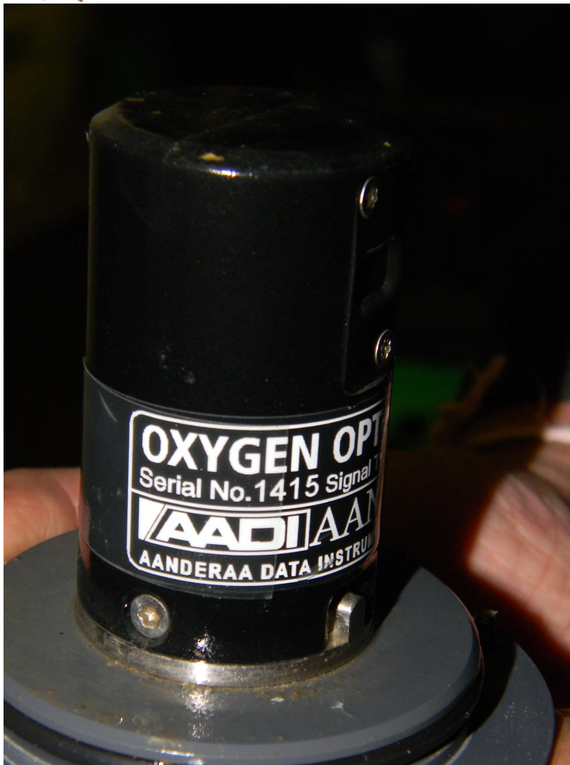
Figure 7: Some minor fouling and sediment within the OPTODE housing.
