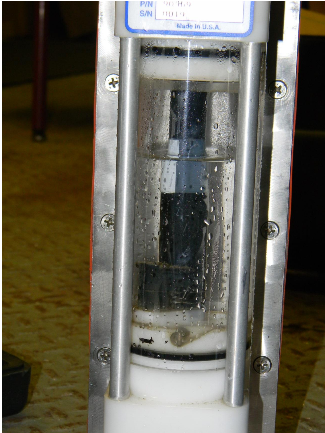
Figure 3: Fouling just starting to be apparent in the CT unit.
