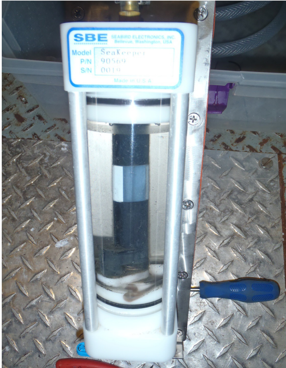
Figure 2: CT Sensor fouling
