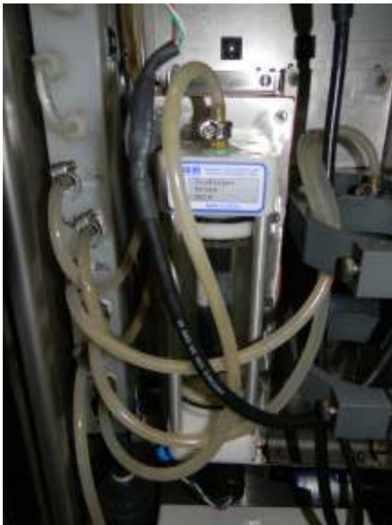
Figure 2: Some Mussels just visible above o-ring on lower end cap of CT unit.
