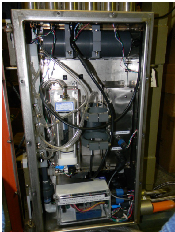
Figure 8: BBFL2 Post-Cleaning; note irregular surface of sensor
