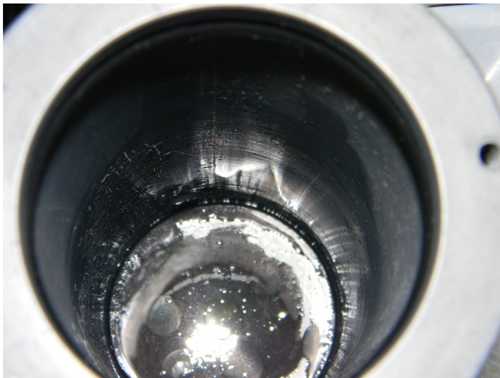
Figure 8: BBFL2 Post-Cleaning; note irregular surface of sensor
