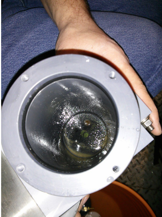
Figure 7: BBFL2 housing prior to cleaning. Note that sediment was NOT on the sensor face prior to removal from system. The housing cannot be kept level and the water must be agitated during removal
