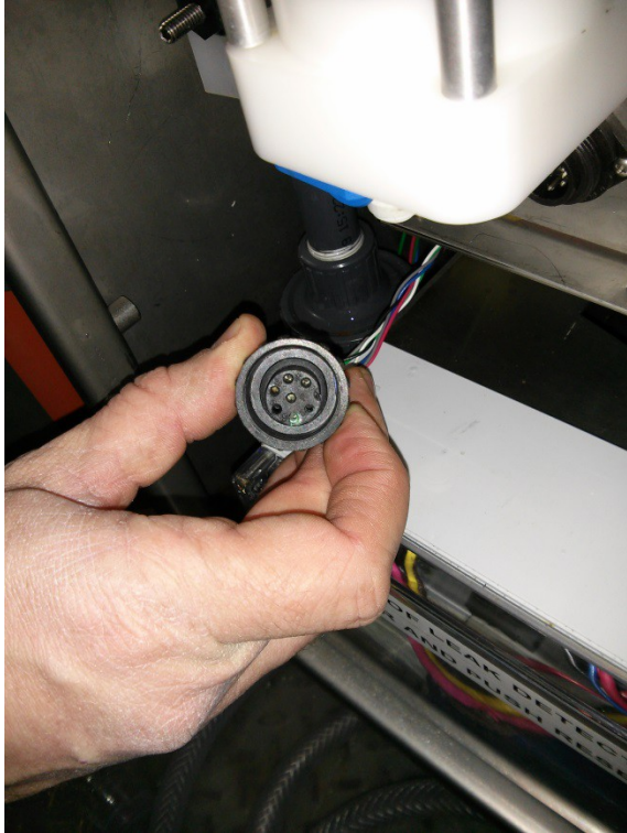
Figure 1: Corrosion evident on connector pin #5
