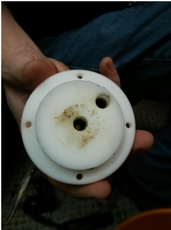
Figure 3: Water evident within housing and on boards
