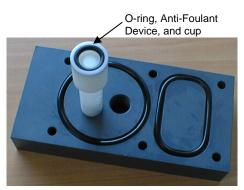
The MicroTSG has an anti-foulant device cup inside the housing. New MicroTSGs are shipped with an Anti-Foulant Device pre-installed in the cup.
