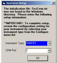
Select the instrument type (SBE 45) and the computer COM port for communication with the MicroTSG. Click OK.
