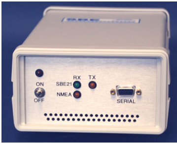
PN 90488 – SeaCAT/Sealogger RS-232 and Navigation Interface Box
