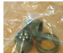
50369 5-pin MS connector assembly (for NMEA Input connector on Interface Box)
