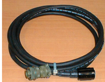
I/O cable (SBE 21 to Interface Box)
