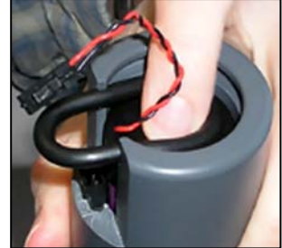
Inserting O-ring into PVC battery case to hold battery in place.
