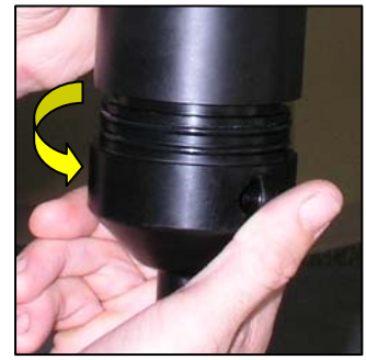
Hand tightening the case
