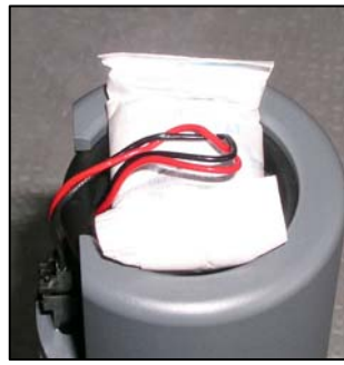
Desiccant pack in place
