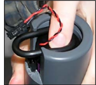
Removing the battery's O-ring
