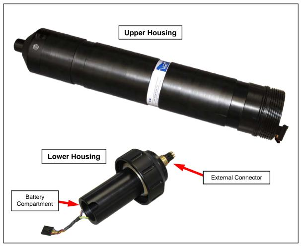
A VR2C-69kHz with lower housing removed.
