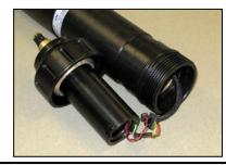
DO NOT impact the threads on the VR2C or they will dent and prevent the VR2C case from closing. See the Trouble Shooting section of the Appendix for tips on thread care.
