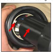
extremely careful to avoid pinching the wiring harness between the upper and lower housings.
