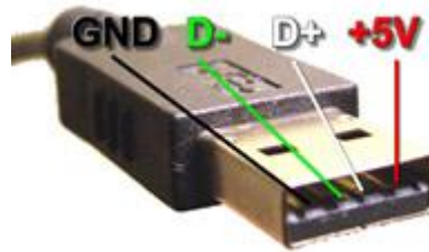
Figure 11-7: USB pin positions
