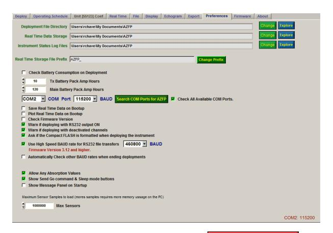
Check your connection by going to the AZFP tab and click on the command button. This will end AZFP deployment if it is deployed and return status information.
