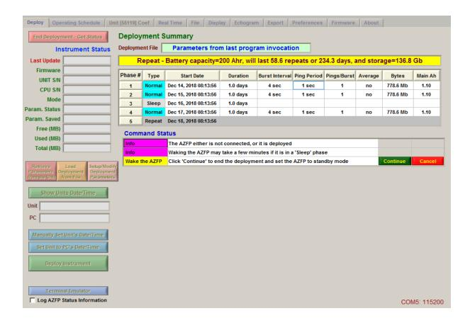
The tab labeled 'Deploy' contains a number of command buttons and sub tabs used to program the unit.
