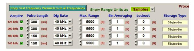
The Copy First Frequency Parameters to all Frequencies command button causes the settings of the first channel to be copied to the rest of the channels.
