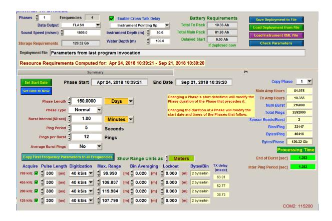
The example below shows the Operation tab with 12 phases. Note the tabs P1, P2.. P12. These tabs contain the settings for the individual phases. These are described in a later section.
