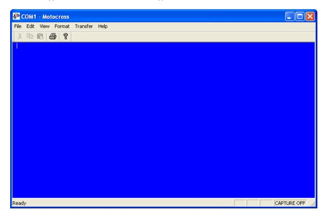
Note in the top left hand corner of the window "COM1 - Motocross" this indicates that the Motocross program is linked to RS232 communications port 1. If this is not the correct port and/or this is the first time Motocross has been launched then the COM port must be set up in the preferences menu. To do so click on the File pull down menu.
