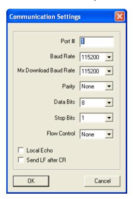
Enter the correct port number. The rest of the settings must be set as shown above.
