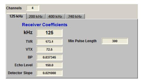
The channels indicator shows the number of acoustic channels installed. There is a corresponding tab for each channel showing the frequency and the calibration coefficients for the channel.
