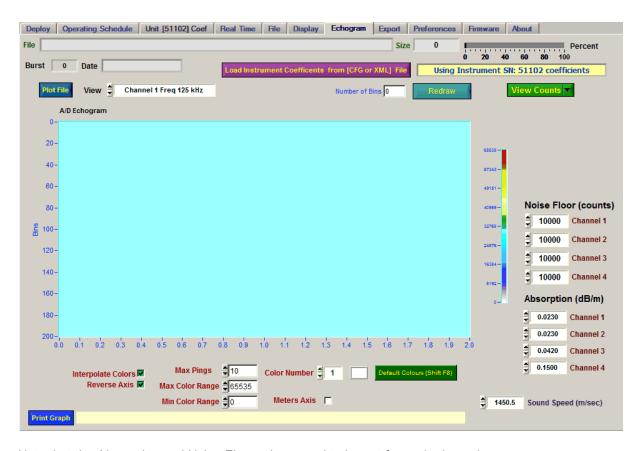
Note that the Absorption and Noise Floor values need to be set for each channel.
