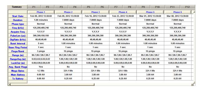
The values in these tables can not be changed on this table. To get to the tab value parameter you want to change select the item by right clicking on it. For example the Pulse Len on Phase 1.
