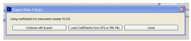
If the user chooses Load Coefficients form CFG or XML File they are asked to load an XML file (created by the instrument during acquisition) or CFG (configuration file) provided by the manufacturer.
