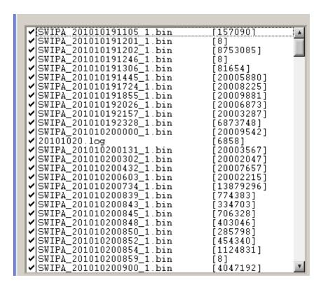
This places a check mark to the left of the file name. Note that this can be manually done by clicking on a file name or passing over the left area with the left mouse button clicked down continually.
