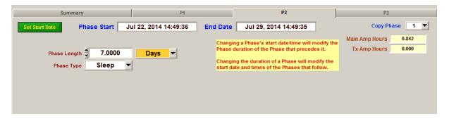
Only the last phase can be a repeat phase. A repeat phase is a phase which switches back to the first phase. Below is an example of a repeat phase.
