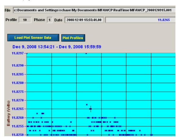
The example above shows the cursor snapped to profile 10 battery voltage data at a value of 11.8265.
