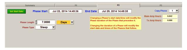
A sleep phase can not be the final phase. AzfpLink will not allow programming of the unit if it is.
