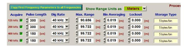
The computation to Meters uses the user selected <u>Sound Speed</u> at the top of the <u>Operating Schedule tab</u>.
