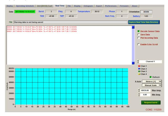
The enables or disables an option to view the profiles being captured by AzfpLink in a scrolling echo-gram.
