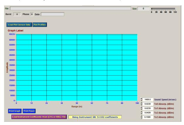
If the unit has calibration coefficients the user should set the absorption values for each channel.
