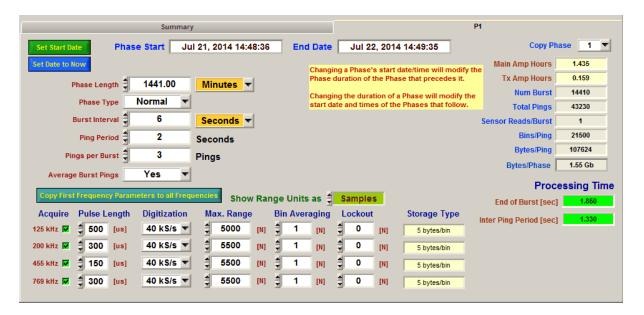
Sleep phases cause the program to end data acquisition and restart it at a later time. The first or last phase cannot be a sleep phase.
