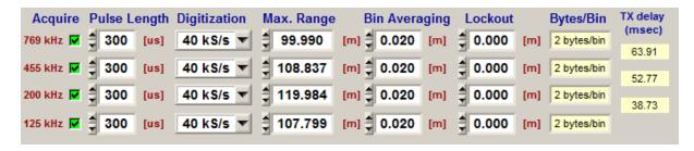
In the above example a 63.91 ms delay is performed after the transmission of the 769 kHz channel, then a 52.77 ms delay after the transmission of the 455 kHz channel and finally a 38.73 ms delay after the 200 kHz channel. Note that the channels are transmitted with the highest frequency first to the lowest frequencies last.
