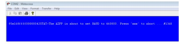
You have 3 seconds to type in three 'x' characters to abort the change of BAUD rates to the higher BAUD rates.
