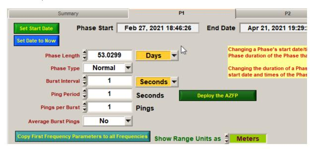
If Burst Mode is not enabled then it is assumed that continual operation is set at the current Ping Period and the burst mode parameters disappear.
