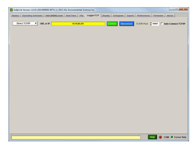
Select the IP address and port number and click connect to connect directly to the AZFP.
