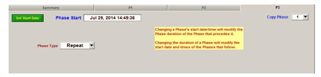
This is accomplished by resetting the Acquisition Start Date to the start date of the repeat phase and then resetting all the start dates of the other phases.
