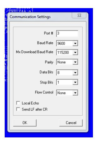
Set the BAUD rate to 9600 BAUD as shown above.
