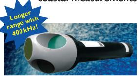
The Aquadopp® profiler measures the current profile in water using acoustic Doppler technology. It is designed for stationary applications and can be deployed on the bottom, on a mooring rig, on a buoy or on any other fixed structure. It is a complete instrument and includes all the parts required for a self contained deployment with data stored to an internal data logger. Typical applications include coastal studies, online monitoring and scientific studies in rivers, lakes, and channels.
