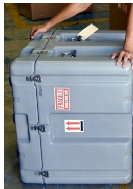
Figure 38. Rotating the Long Ranger / QuarterMaster Shipping Case During Compass Calibration
