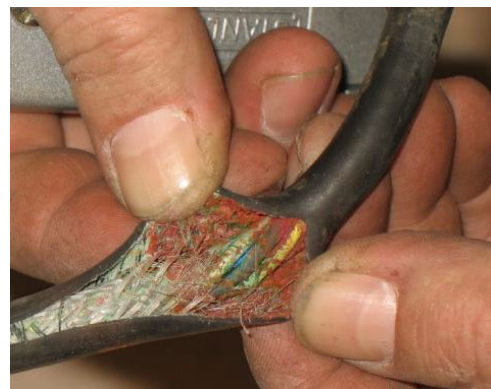
Figure 11. Do not use Zip-Ties Directly on Cables
