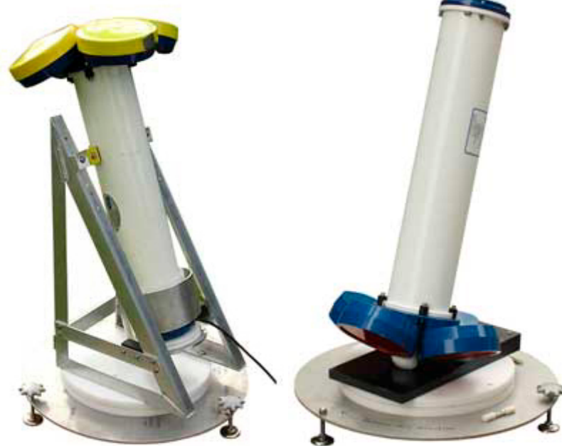
LR-1A is shown with Teledyne Long Ranger loaded for a UPWARD Profile Calibration
