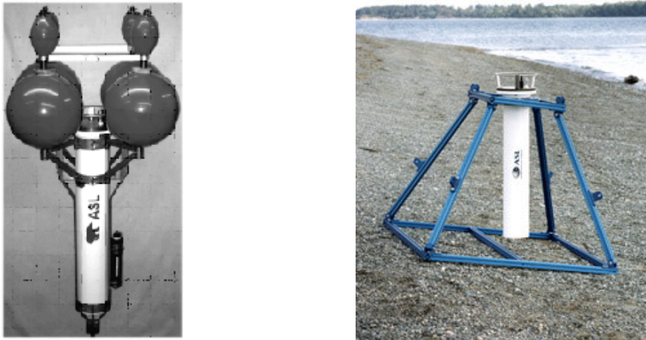
Figure 1. AWCP in (a) a mooring cage and (b) in a bottom frame
