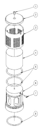
Figure F-2: Biofouling Guard Exploded Assembly
