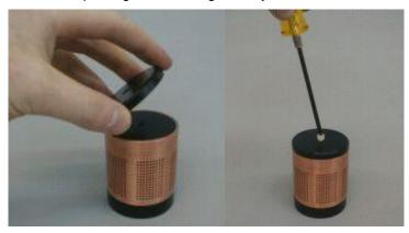
Figure F-7: Attach the end cap
