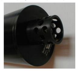
Figure A-13: Standard Probe Guard Attached
