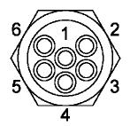
Figure A-7: MCBH6M Bulkhead, Male Face View
