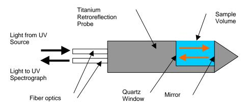
Figure A-3: Seawater Sample Illumination
