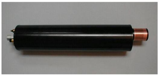
Figure F-10: The ISUS with Biofouling Guard
