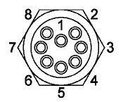
Figure A-9: MCBH8M Bulkhead, Male Face View
