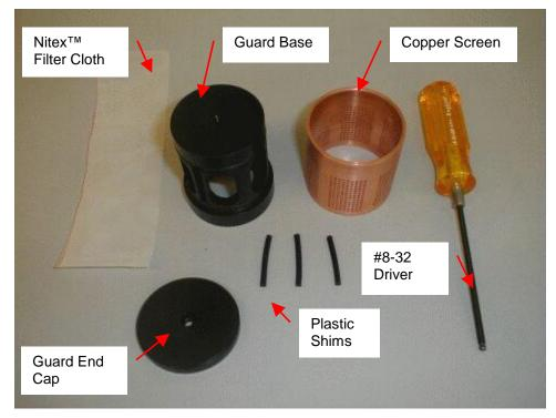
Figure F-1: Biofouling Guard Components
