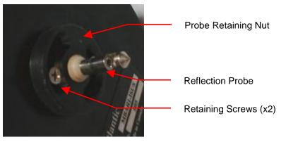
Figure A-12: Reflection Probe
