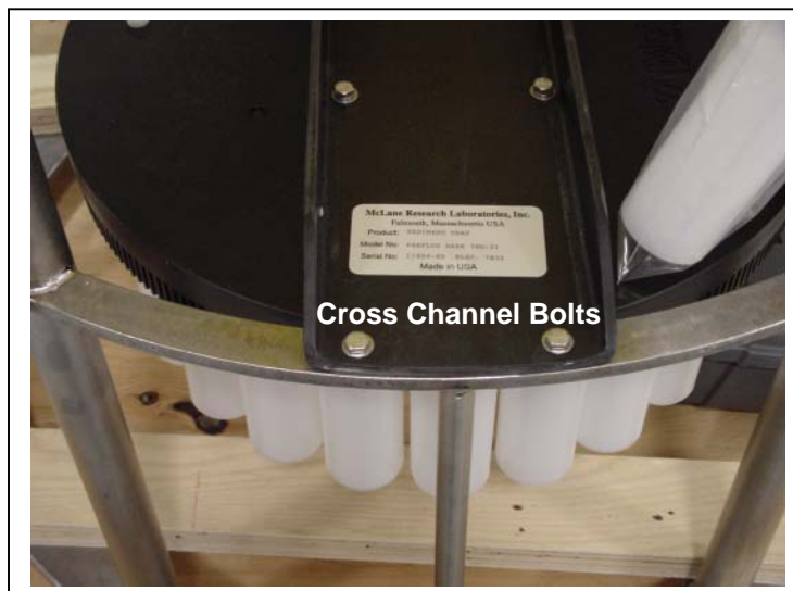
Figure C-3: Remove Cross Channel From Frame
