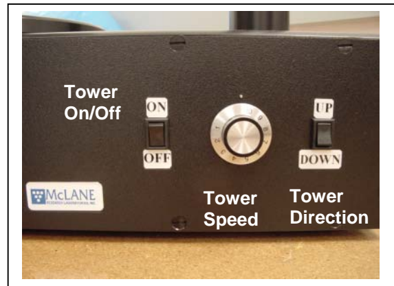
Figure D-3: WSD-10 Tower Controls
