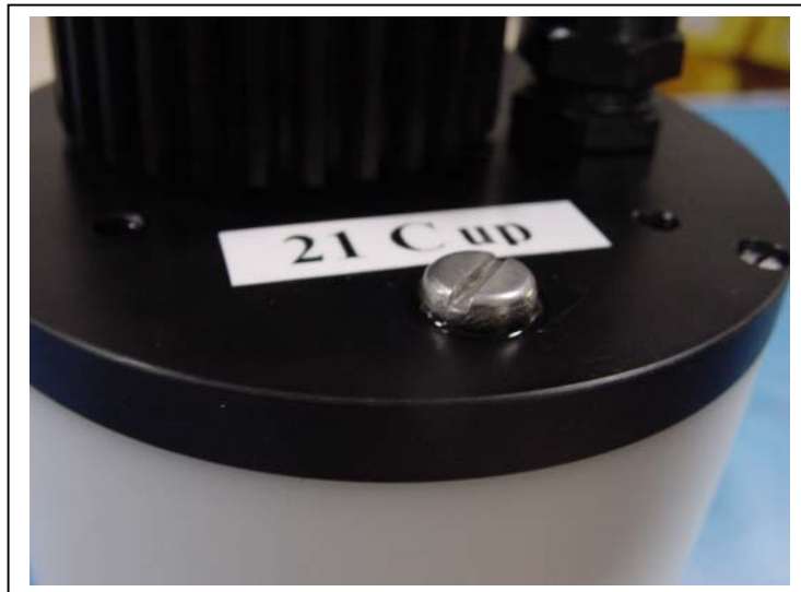
Figure 4-6: Oil Around Fill Hole Screw
